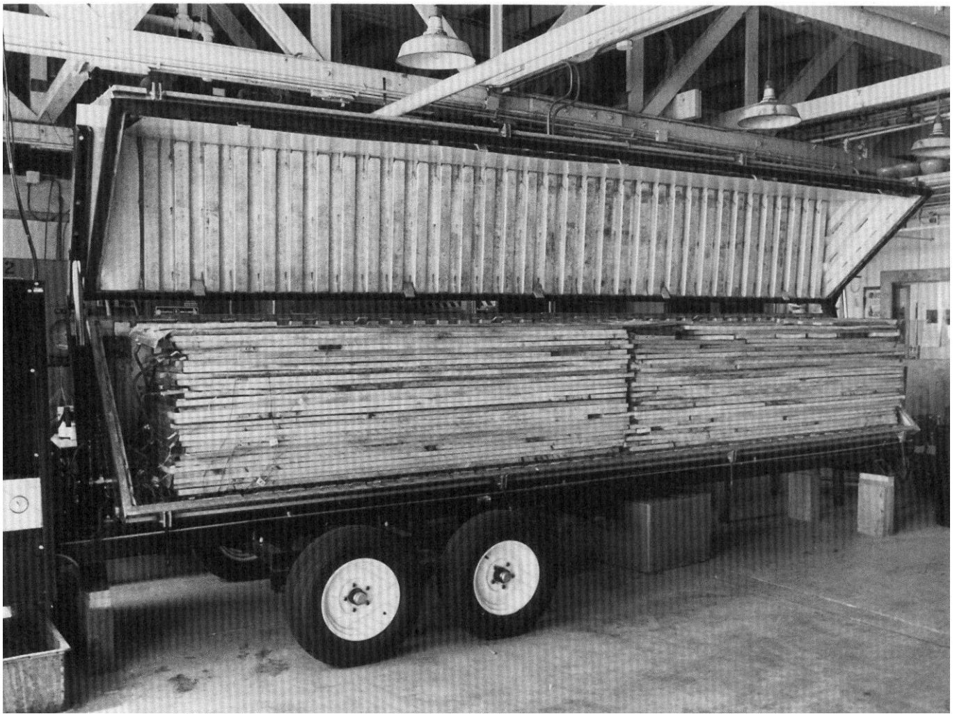
Figure 2-27—Vacuum-kiln type in which heat is supplied to the lumber by contact with electrically heated blankets. (M85 0351-10)
