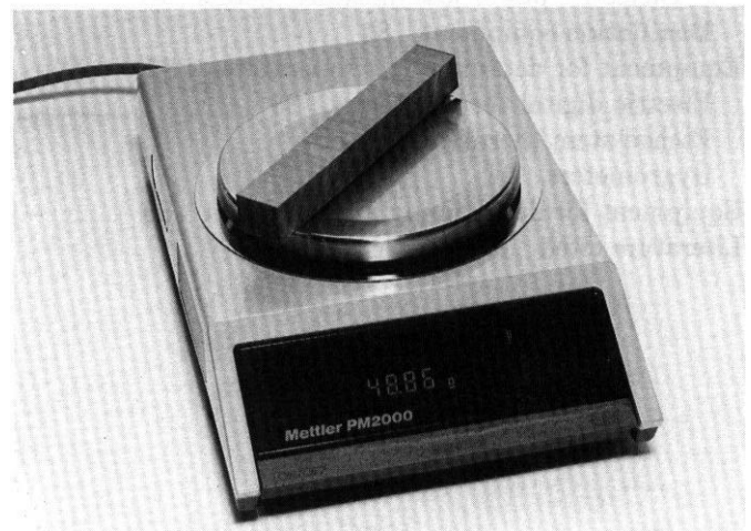
Figure 3-2 —Electronic top-loading balances suitable for weighing small moisture sections. (M87 020, M87 0175)
