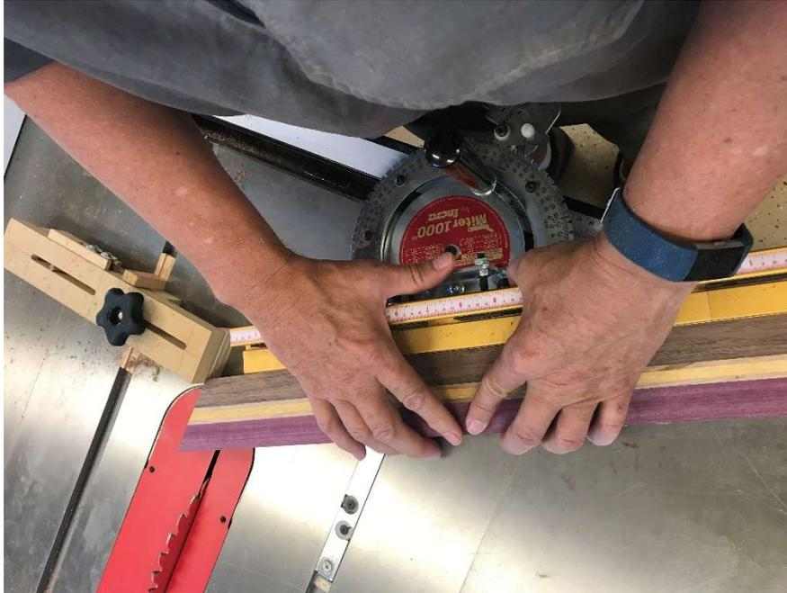
3. Layout the strips you just cut in pairs. Flip one strip in each pair to make a chevron. Glue two strips together and clamp. Alignment is critical. Make a few more chevrons than you'll need for your feature ring. Then you can choose the best-looking ones for use in your feature ring.
