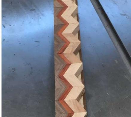
7. While still attached to the base MDF, run the assembly through the drum sander. Then, remove the chevrons from the MDF.
