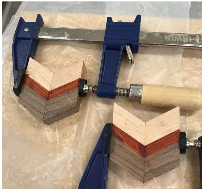
4. Each chevron needs to be trimmed to remove the 'pointed' parts of the chevron assembly. Malcolm Tibbetts suggested a method that produces uniform segments. Get a piece of plywood or MDF that is as wide as your chevron assemblies and long enough to hold all of them side by side. Put two strips of double-sided tape running the length of the MDF, placing the tape wide enough to stick to the main part of the chevron and also the portion of the tips that will be removed. (This
